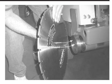
Figure 11. Aligning Flange Pin Through Blade
